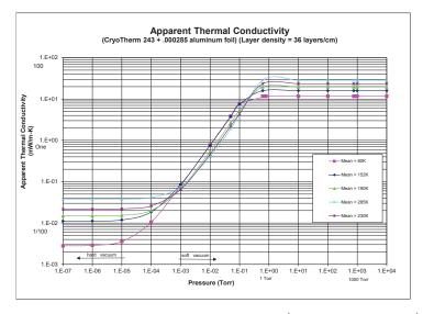
Note: The thermal performance graph represents the historical CRS Wrap (CryoTherm 243 and Aluminum foil). The CRS Wrap with Biosoluble CryoTherm is expected to offer the same performance.
