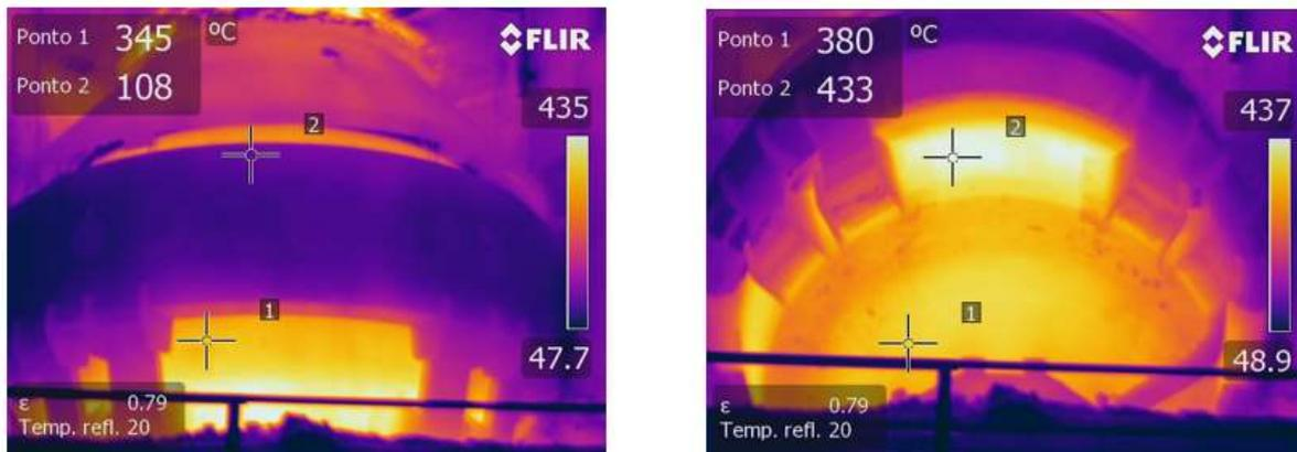
**Figure 9 – Thermography performed on BOF with 400 heats.**
