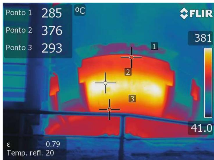
**Figure 10 – Thermography of BOF#4 with 4000 heats.**
