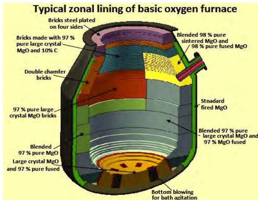
Figure 1 - Schematic representation of the converter (5)
