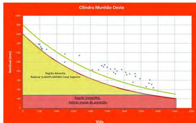
Figure 11. Trunnion wear curve.
