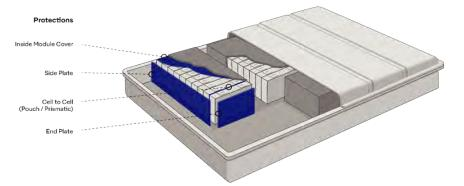
Alkegen offers many UL listed FyreWrap® product forms and FyreWrap fire protection materials for passive fire protection applications.
